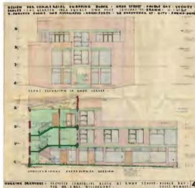
Figure 9: Evan's Knox Street elevation and section of the proposed "shopping block" at No 21 Bay Street.
